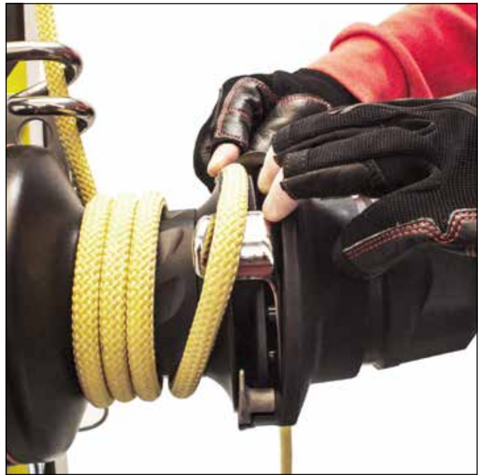
4. Fit the rope into the rope grab. Raise the cover to make this easier. Position the rope inside the stopper.
