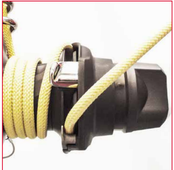
4. Fit the rope into the rope grab. Raise the cover to make this easier. Position the rope inside the stopper.
