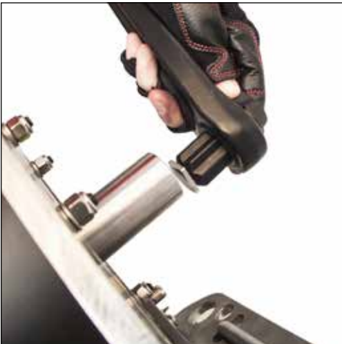
6. Insert the winch handle into the socket.
