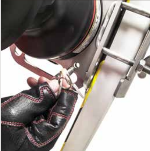
5. Fix surely the plate with the self-locking nut.
