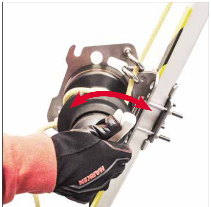
Check that the rope grab knob is working by rotating the knob and releasing it.
