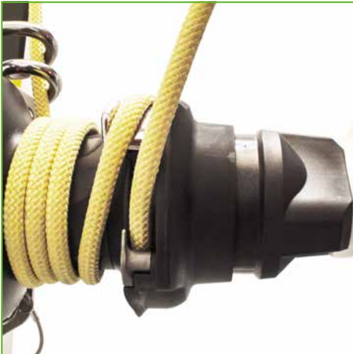
3. Pull rope through to take up any slack, then pass the rope on the stripper arm by winding rope clock-wise and pulling tight to engage.
