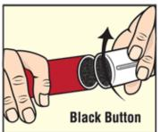
**3.** Hold away from face while activating Chimfex by lightly scratching black button with the cap.
