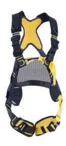
A very light and compact fall arrest harness with 2 connection points: 1 sternal and 1 dorsal. Quick release buckles to the thighs and a foamed back allow a quick sitting. Versatile because it can be combined with a work position belt.
