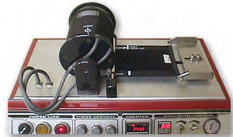
Cuff hook and loop adhesive test
