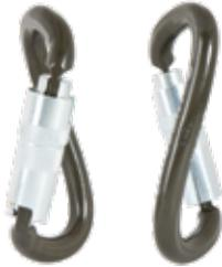
The CMC DNA ANSI Carabiner has a helical-shaped connector with a twisted carbon steel body and circular bar. This twist allows for a 90° rotation of any connected device, optimizing alignment and assisting with offset load management. Excellent choice for the Double CLUTCH.
