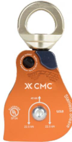
By combining a swivel with the pulley, the overall system length is minimized, increasing travel. The patented pivoting side plate allows a rope to be quickly inserted.
