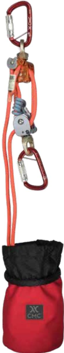
The AZTEK ProSeries LT (Load Tender) is a more compact version of the AZTEK ProSeries System on page 114. Reflecting attention to detail, the LT system includes 8.5 m (28 ft) of 8 mm AZTEK ProSeries Cord that can extend the set-of-fours up to 6 feet, providing a 4:1 or 5:1 mechanical advantage with an MBS of 38 kN (8,542 lbf). The LT System includes two ProTech™ Auto-Lock Carabiners with removable keeper pins for attachment to swivel ends.
