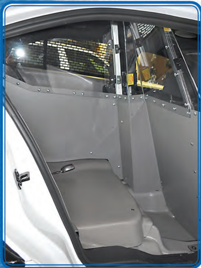
A SINGLE CELL, SHOWN HERE IN A PI SEDAN, PROVIDES A SECURE TRANSPORT AREA FOR EVEN LARGER PRISONERS.
