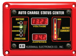
Status Center Display in Watertight Case 091-194-IND-WT-XX
