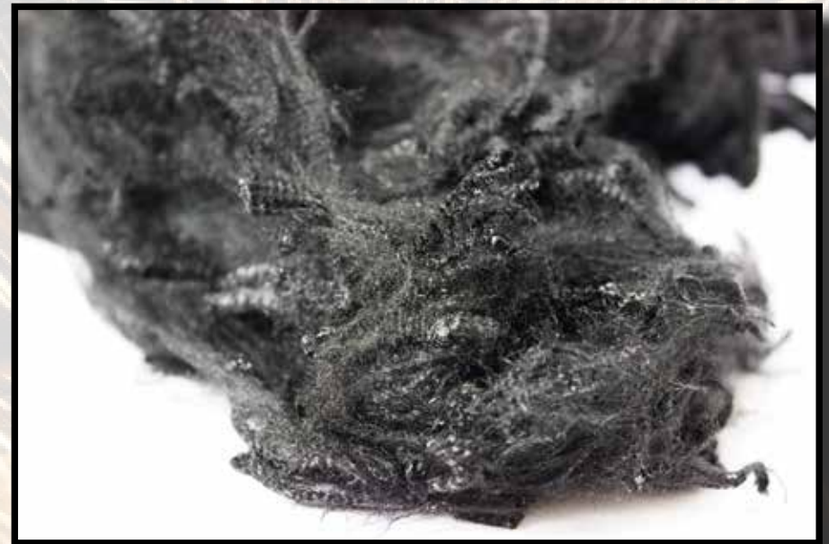
OPF (Oxidized Polyacrylonitrile Fibers) provides increased protective textile characteristics such as high thermal stability and low thermal conductivity.
