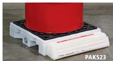
Deck captures small spills and leaks. Bladder stays rolled up behind trap door until sump is full and then deploys automatically.
