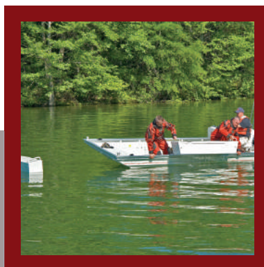
Floating Sea Boxes Removable floating boxes can be used as flotation/rescue devices or deployed to create more working area.
