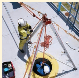
Tripod as High Directional with remote haul system
