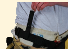
Harness keeper tab snaps around waist belt of harness.
