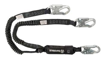
**PRO 6' Stretch Energy Absorbing Lanyard:** 12' FF Dual Leg, Snap Hooks
