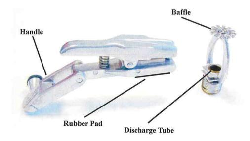
After inserting jaws, fold handle up. This compresses rubber piece over discharge shutting off water.
