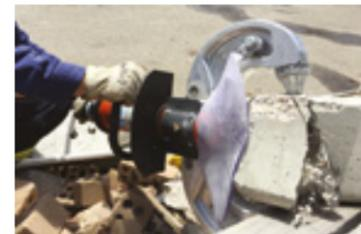
A perfect combination: crushing concrete with the CC 23 and cutting re-bar with mini cutter CU 4007 C or SMC 5006
