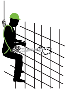
FIGURE 7 - PROPER USAGE WHEN POSITIONING ON VERTICAL REBAR
