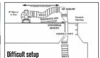
The LFR connects directly to the fan using a built-in strap. Meanwhile, the saddle duct requires setup of multiple components, including manhole lid.
