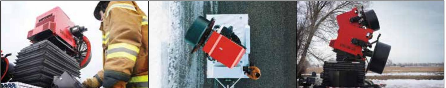
**3 Rotate, Raise and Tilt:** The Electric Turntable rotates the fan up to 270°; the Scissor Lift extends the SVU up to 30' in the air and tilts 20° up and down
